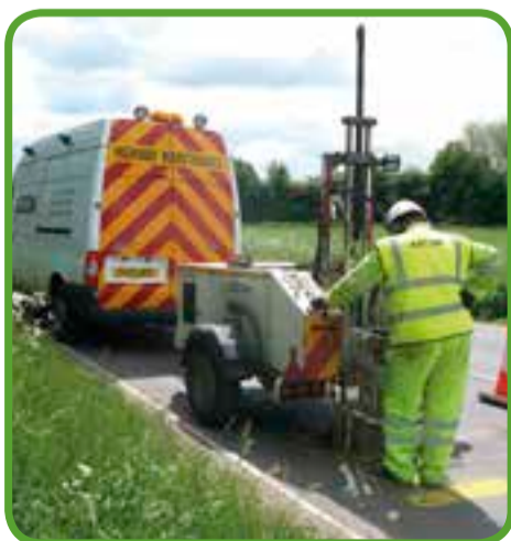
Coring and material testing for Nottinghamshire
