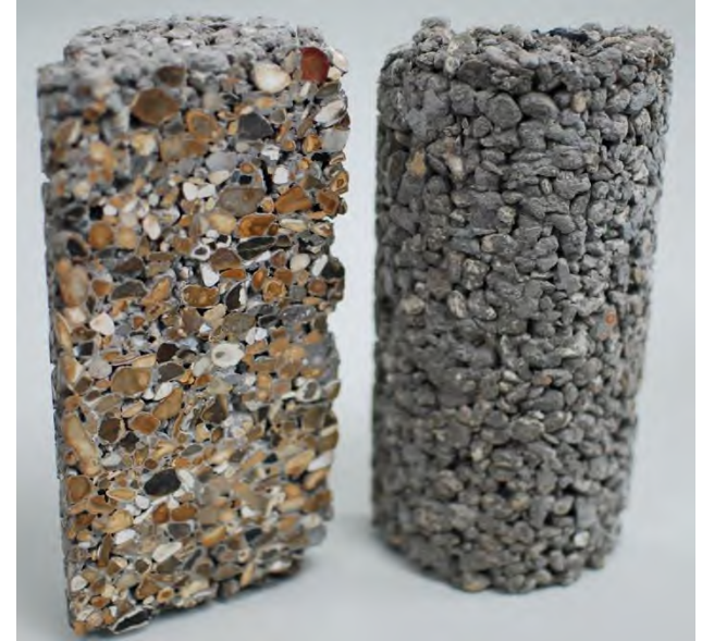
Conventional permeable concrete pavement cross-section
