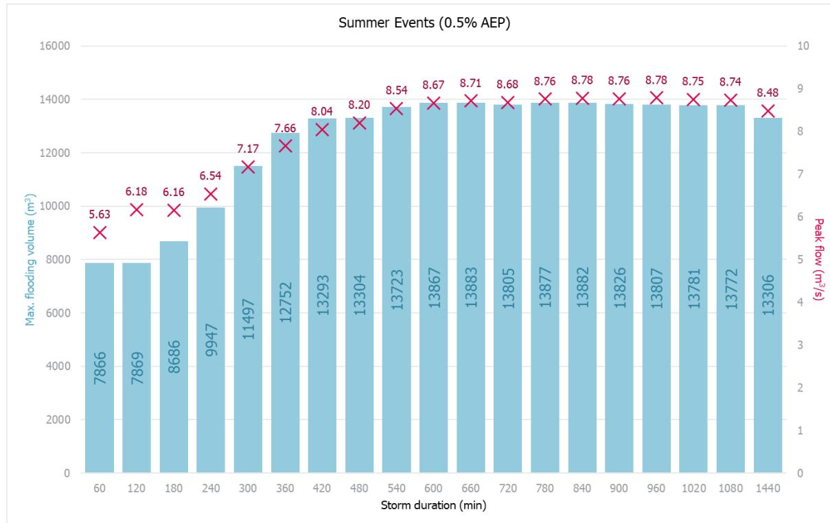
Hydraulic analysis and inundation mapping has been carried out using an integrated catchment model which includes watercourses, urban drainage network and their interactions, for the following return periods:
