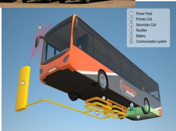
Electric bus service: induction charging
