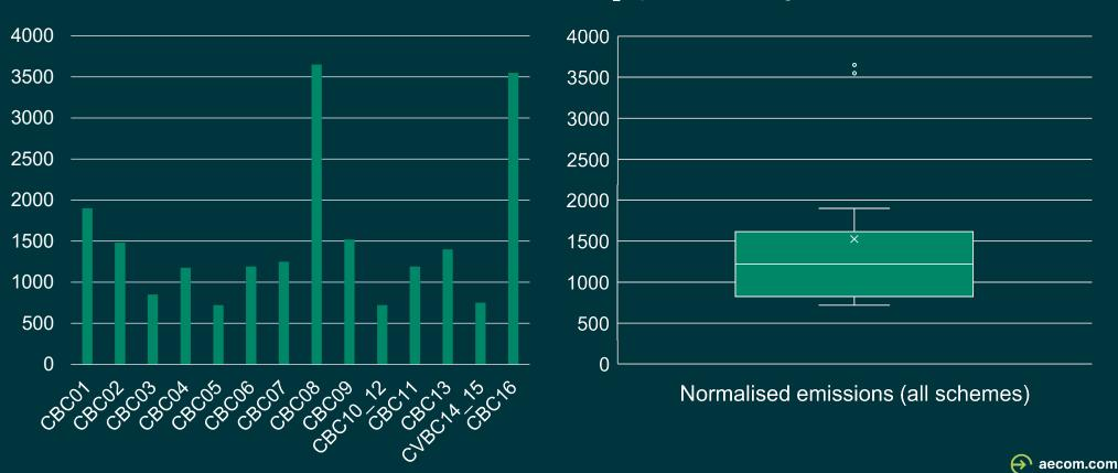
Normalised Carbon Emissions – Tonnes CO<sub>2</sub>e per KM – Design Scenarios
