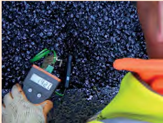
Figure 1: Recording the temperature of Low Temperature Asphalt (LTA)
